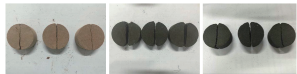
图 1 天然砂岩试样及 3D 打印试样巴西劈裂破裂 Fig. 1 Brazilian test of natural sandstone samples and 3D printed samples
